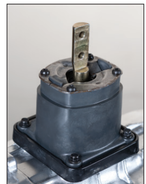
S10 Manual Shift Lever Adapter Installed in Factory Shifter.
