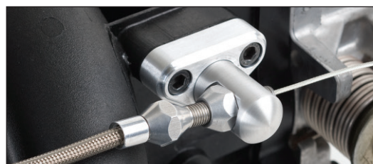
LS1 Throttle Cable Bracket - Single Stud Shown
