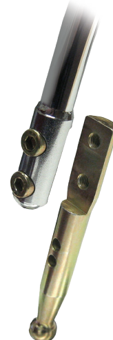
S10 Manual Shift Lever Adapter Installed in Factory Shifter.
