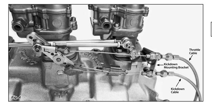
Throttle Cable and Kickdown Cable not included. Both are available separately. The Kickdown Mounting Bracket is part of the Kickdown Kit.
