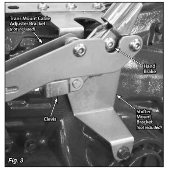
NOTE: To release the Hand Brake, you must pull up slightly on the handle while depressing the release button. Keep the release button depressed while you lower the handle to it's at-rest position.
