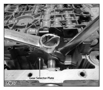
Step 13: NOTE, AODE and 4R70W Only: Install the new Lokar Flange onto the Selector Shaft. If using the original selector shaft, use the original nut or bolt to retain the flange. If using the Lokar Selector Shaft, install the supplied 3/8"-16 x 3/4" lock bolt into the Selector Shaft to retain the flange
