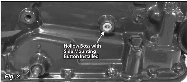
Hollow Boss with Side Mounting Button Installed
