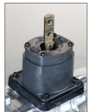
S10 Manual Shift Lever Adapter Installed in Factory Shifter.
